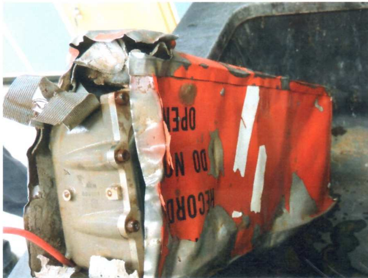
Figure 3. Damage to left side and front of recorder.
