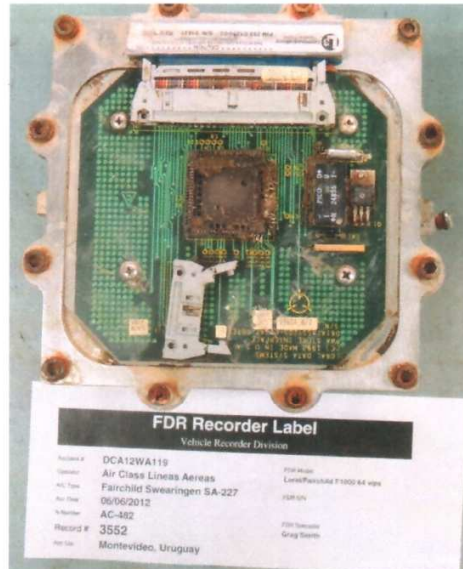
Figure 7. Disassembled memory module.
