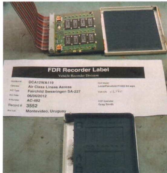
Figure 9. New connector crimped onto ribbon cable.
