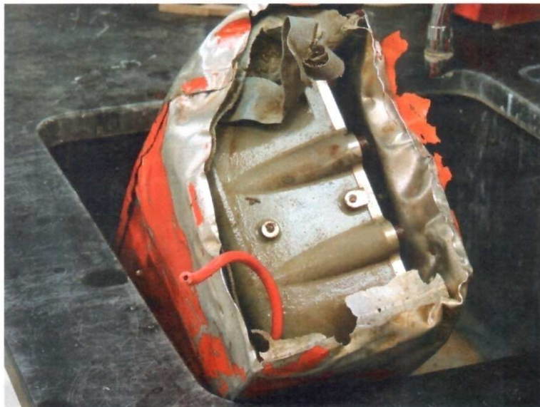
Figure 1. Damaged front end of flight recorder.
