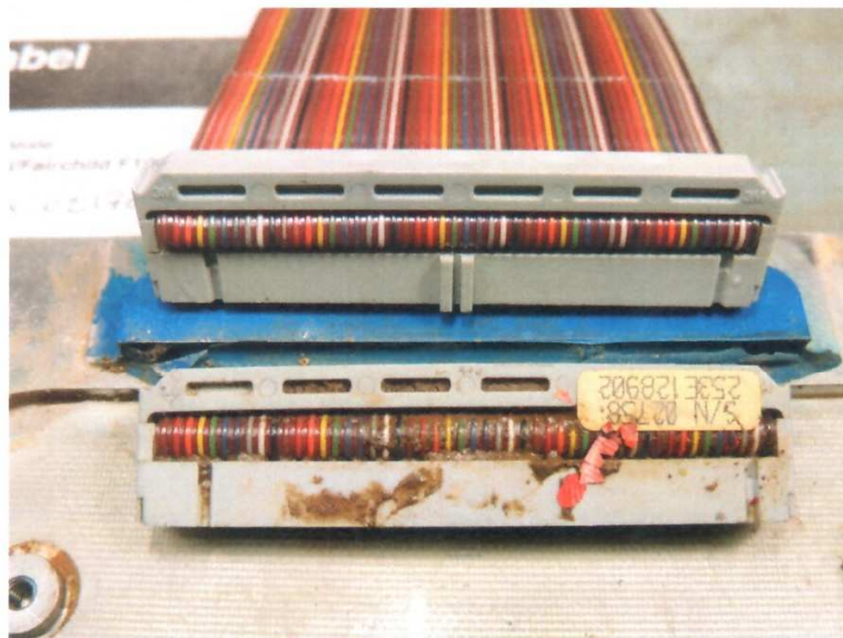
Figure 9. New connector crimped onto ribbon cable.
