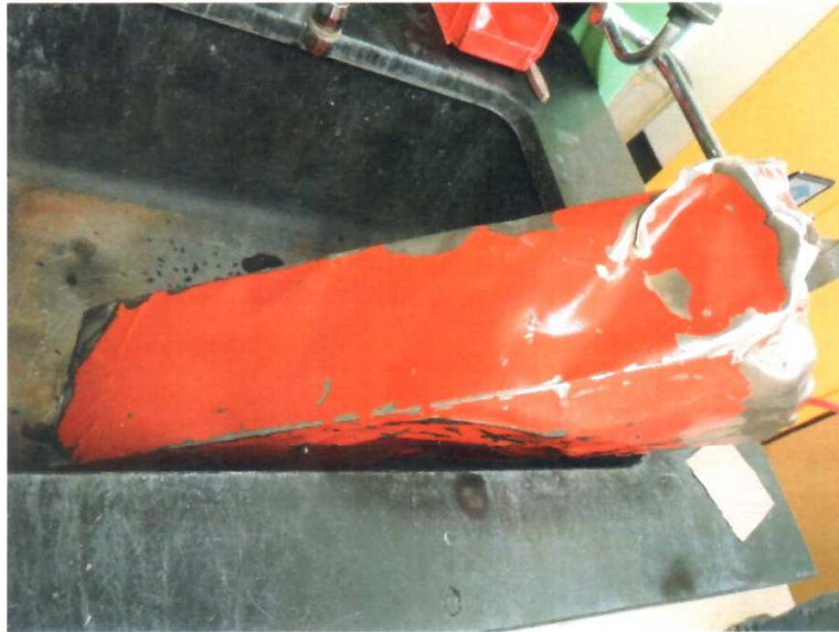
Figure 3. Damage to left side and front of recorder.
