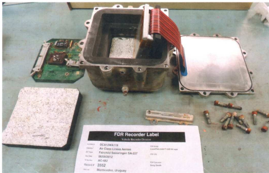
Figure 7. Disassembled memory module.
